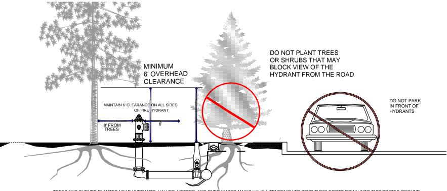
TREES AND SHRUBS PLANTED NEAR HYDRANTS, VALVES, METERS, AND OVER WATER MAINS HAVE A TENDENCY TO SEND THEIR ROOTS DOWN INTO THIS SOFTER GROUND. THESE ROOTS CAUSE MAINTENANCE PROBLEMS FOR THE CREWS, AND CAN END UP BREAKING WATER MAINS AND INTERFERING WITH THE OPERATION OF THESE CRITICAL COMPONENTS OF THE WATER SYSTEM. PLEASE AVOID PLANTING TREES AND LARGE SHRUBS WITH-IN 8 FEET OF ANY OF THESE INFRASTRUCTURE ITEMS.
